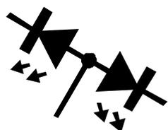
3-lead bicolour LEDs are available in common cathode and common anode varieties. The *DCA Pro* supports both types.
