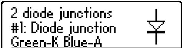
The details for the first diode are then displayed (Diode #1). In this example, the Green test clip is on the Cathode of diode #1 and the Blue test clip is on the Anode.
