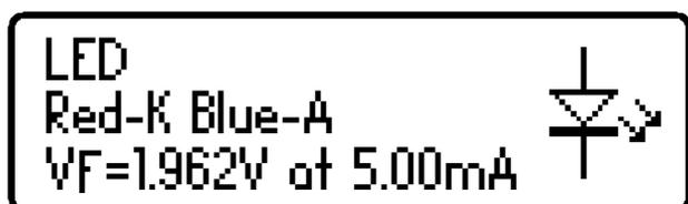
In this example, the Red test clip is connected to the LED's Cathode (negative) and the Blue test clip is connected to the Anode (positive).
