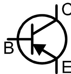
Bipolar Junction Transistors are simply “conventional” transistors, although variants of these do exist such as Darlington, devices with free-wheeling diodes, resistor shunted types and combinations of these types. All of these variations are automatically identified by the *DCA Pro* and their schematic symbol display on the screen. Both NPN and PNP types are supported.
