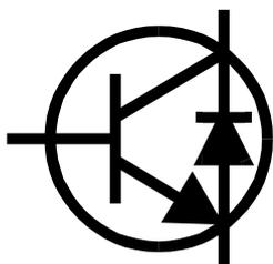
For NPN transistors, the anode of the diode is connected to the emitter of the transistor. For PNP transistors, the anode of the diode is connected to the collector of the transistor.
