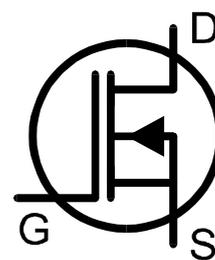
The fairly rare Depletion Mode MOSFET is very similar to the conventional Junction FET (JFET) except that the gate terminal is insulated from the other two terminals. The input resistance of these devices can typically be greater than 1000MΩ for negative and positive gate-source voltages.
