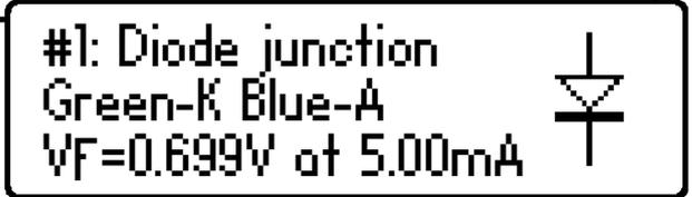
The details for the second diode are then displayed (by briefly pressing **scroll-off**):
