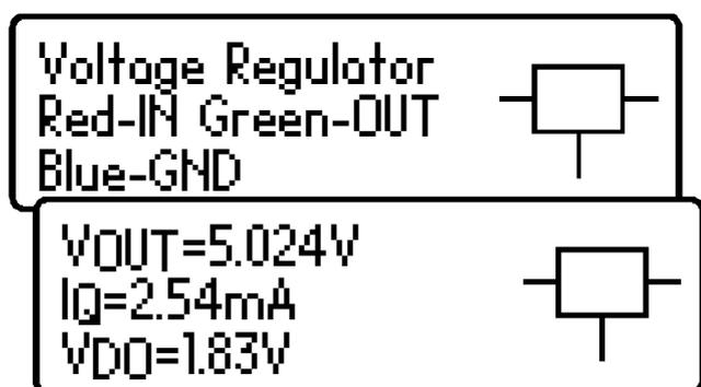
When a regulator is identified, its pinout, output voltage, quiescent current consumption and drop-out voltage are displayed.
