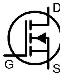
MOSFETs of all types are sometimes known as IGFETs, meaning *Insulated Gate Field Effect Transistor*. This term describes a key feature of these devices, an insulated gate region that results in negligible gate current for both positive and negative gate-source voltages (up to the maximum allowed values of course, typically  $\pm 20\text{V}$ ). IGFETs are not to be confused with IGBTs (Insulated Gate Bipolar Transistors), these are dealt with in a later section.
