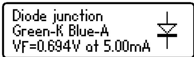
In this example, the Cathode (symbol of K) is connected to the Green test clip and the Anode (symbol of A) is connected to the Blue test clip,
