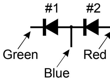
In the same way as the single diode analysis, the forward voltage for each diode is measured for a nominal test current of 5mA.
