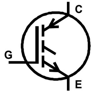
IGBT is an acronym for Insulated Gate Bipolar Transistor.
