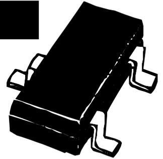
The *DCA Pro* will identify multiple diode junctions between the probes. For three terminal devices such as SOT-23 diode networks, all three test clips must be connected.
