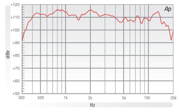
Frequency response measurement taken on axis with 1w signal at distance of 1M using FANE FH-2450 horn
